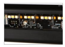
32 state-of-the-art low voltage LEDs give exceptionally bright and even illumination over the entire score. LEDs are virtually indestructible and never wear out, so you'll never again have to change a bulb in the middle of a performance.
