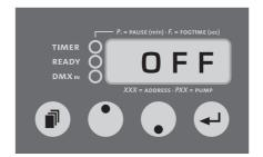
Fig. 4: Display shown for switching off the device
