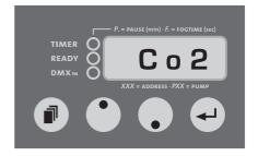
Fig. 3: Display shown when the CO2 is expelled
