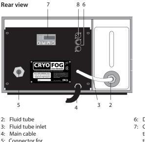
5: Connector for liquid CO2-tube
