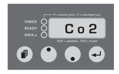
Fig. 3: Display shown when the CO2 is expelled
