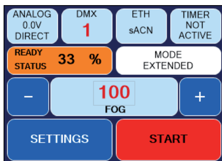
Fig. 1: Machine not ready
