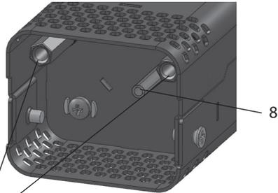
10: Connecting pins for vaporizer
