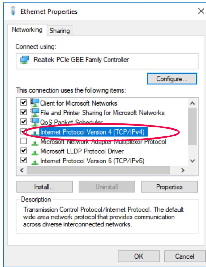
5 Enter the network configuration as shown in the following example and accept the changes:
