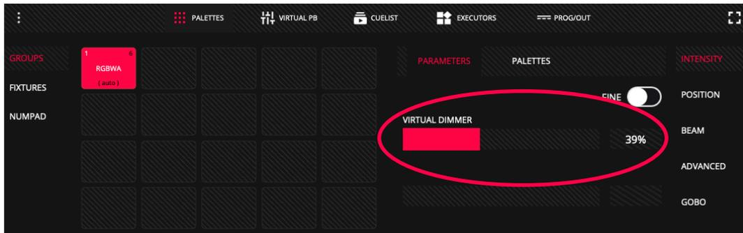
This is where Virtual Dimmer comes in. Having patched our example of a 5-channel RGBWA LED PAR, we can also assign a Virtual Dimmer. This is not another DMX channel, in fact no additional DMX channels are sent from LightShark. Instead, the Virtual Dimmer is a concept that allows fixtures to behave as if they had their own intensity channel that controls the overall brightness and can make use of the Dimmer effect.
