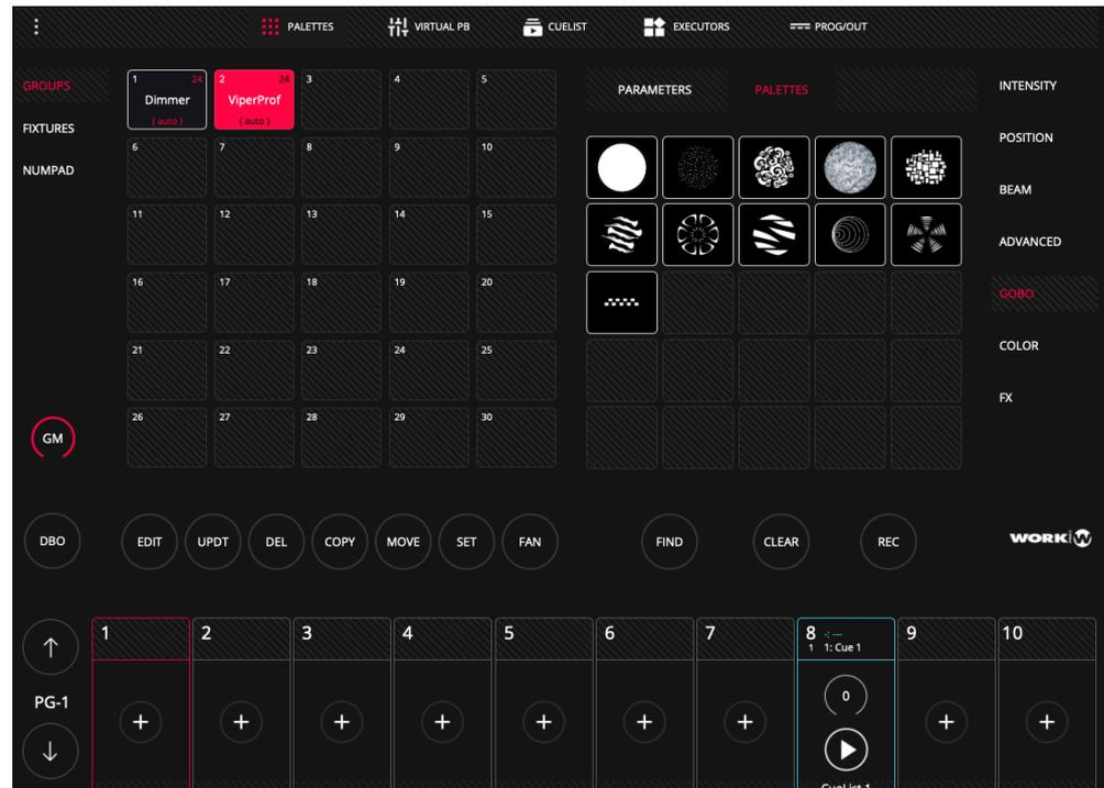
LightShark displays up to 25 palettes simultaneously, it is possible to perform vertical scrolling as in the parameter window to access more palettes.
