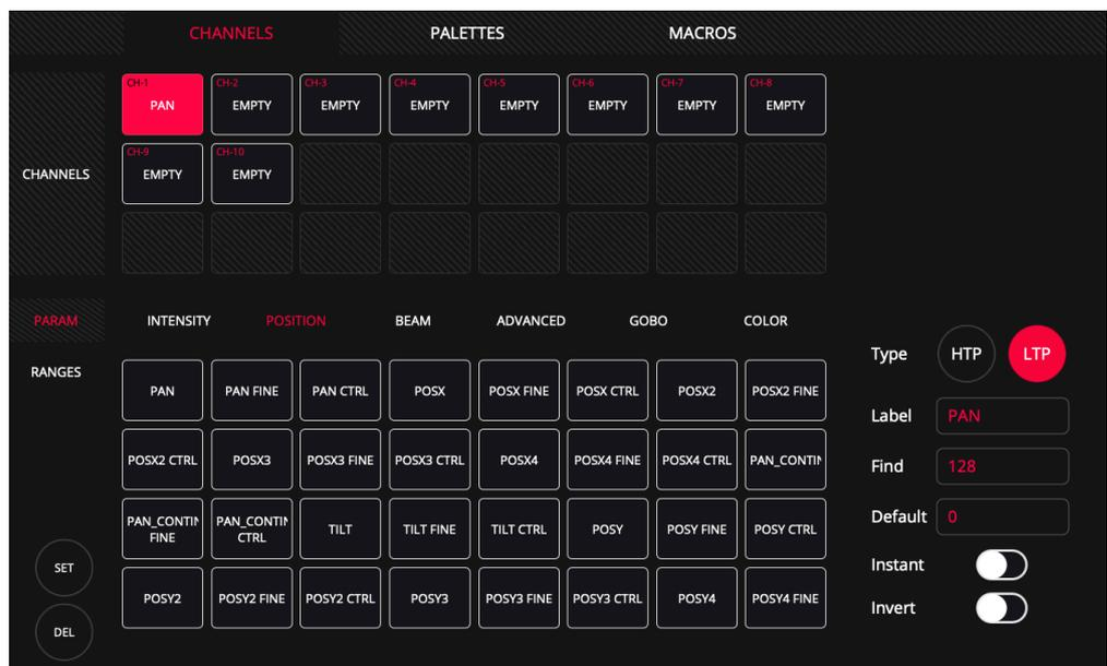
Selecting a lightShark parameter will autocomplete the Channel Type ( HTP or LTP), Label, Find value and Default value. It is possible to configure the channel as "INVERT" or "INSTANT".
