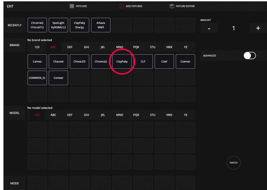
Selecting a manufacturer in the "MODEL" section will display that manufacturer's alphabetically filtered fixtures.
