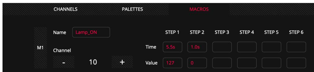
In this example the macro will send a value of 127 to the device for 5.5 seconds and then reset the channel to 0.
