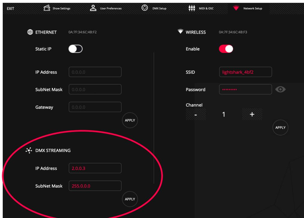
Once the necessary changes have been made, press the "APPLY" button to save the changes. LightShark will restart, loading the new settings at startup.
