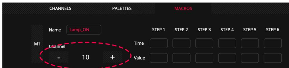
**11** Define the values that the channel must have along the time period for the macro to be executed correctly.
