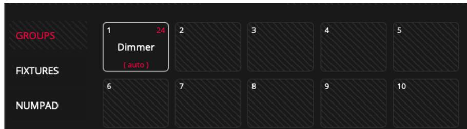
**7** Select the fixture group (or individually in the "FIXTURES" view) and select "INTENSITY" in the parameter area:
