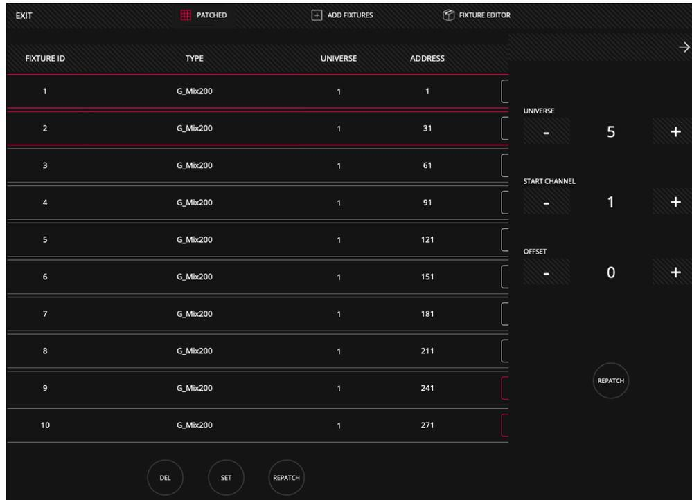
**4** Set the new fixture address and press the "PATCH" button.
