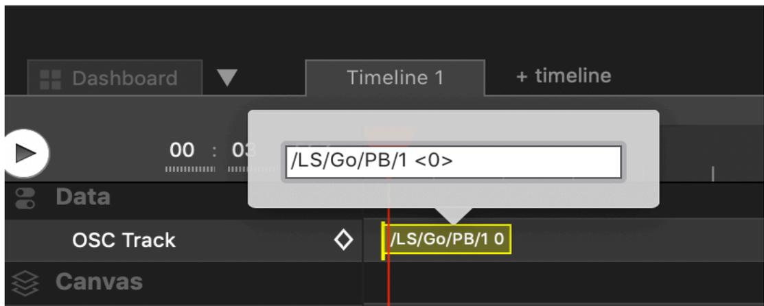
Note that actions in LightShark are performed by releasing the button, so the message is sent on `<0>` value instead of `<1>`.
