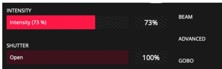
The values included in the programmer are represented in light red, the rest of the values that are not added in the programmer are represented in dark red.
