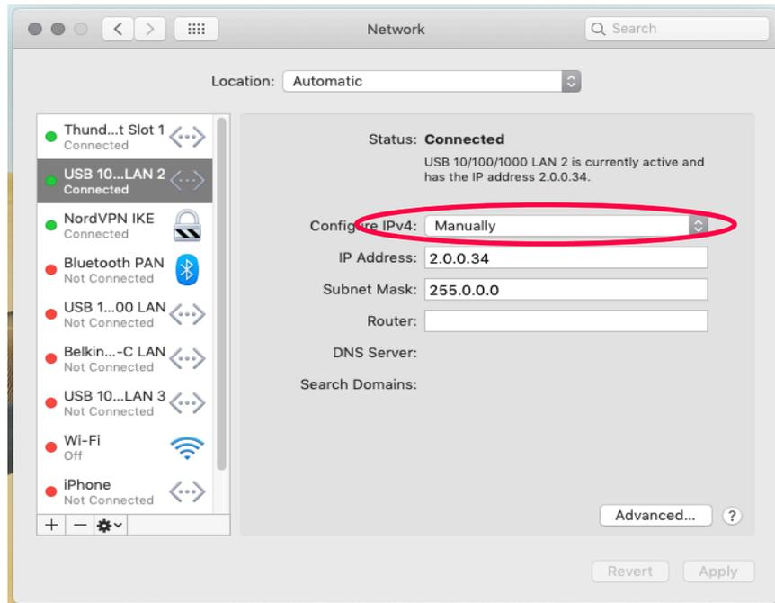
4 Then set the IP address and Subnet Mask as in the following example:
