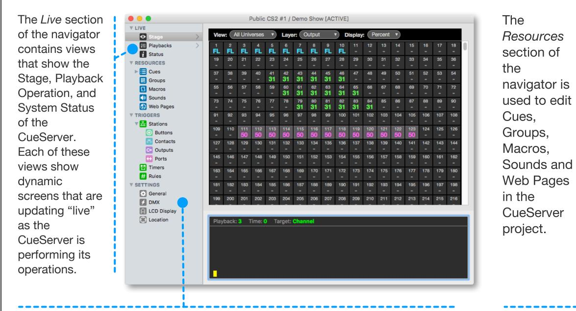
The Settings section is used to edit DMX resources, universe and playback settings, LCD Display and Location settings.
