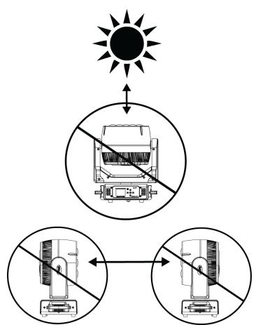
DO NOT EXPOSE THE FIXTURE AND/OR FRONT LENS OPENING TO LIGHT BEAMS FROM DIRECT SUNLIGHT, OTHER LIGHTING MOVING HEAD FIXTURES, AND LASERS WHILE UNPACKING, INSTALLATION, USE, AND EXTENDED IDLE TIMES OUTDOORS. DO NOT FOCUS A LIGHT BEAM FROM ONE LIGHTING FIXTURE DIRECTLY TOWARDS ANOTHER.
