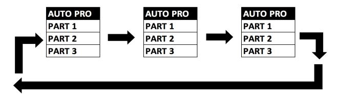
The Secondary unit receives data from the Primary unit according to the group which the Secondary unit was assigned to. If e.g. a Secondary unit is set to **"Secondary 1"** in the menu **"Set to Secondary"**, the Primary unit sends **"Auto Program Part 1"** to the Secondary unit.
