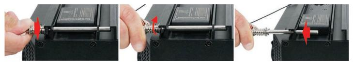
1. To remove spring-loaded locking-pin, compress the spring enough to clear the rail, rotate ring to vertical orientation (stepped rail-block to a horizontal orientation), and pull pin straight out.
