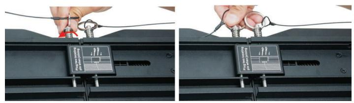
6. Compress the spring of the second locking-pin and rotate the ring 90° to lock it into the rail.
