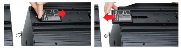
3. Press-click the locking pin abutment block to release the spring-loaded locking mechanism. This pops the abutment block out towards the adjacent fixture.
