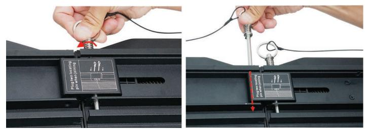
5. Compress the spring of the first locking pin and rotate the ring 90° to lock it into the rail. Insert and lock a second locking-pin through the second set of aligned holes. Ensure that the stepped rail-block of the locking-pin is horizontally aligned with rail slot to pass it through rail slot.
