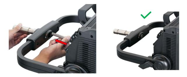
3. Thread the junior pin bolt in through the underside of the mounting yoke, making sure that the bolt engages the threaded hole in the junior pin. Tighten securely with a 10mm hex key. The junior pin is now ready for attachment to a clamp or stand.
