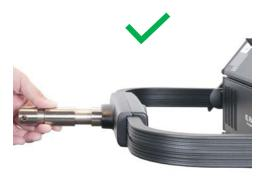
2. Locate the notched face of the junior pin and hold it against the clamp mounting point located on the top side of the yoke. The notched surface of the junior pin must sit flush against the matching groove on the surface of the clamp mounting point.
