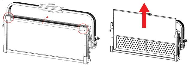
2. Slide the Intensifier Lens into the slot. Please note that the Intensifier Lens is NOT reversible. The forward-facing side of the Intensifier Lens should have a slight ridge in the lens frame, while the rearward-facing side should have a smooth lens frame.
