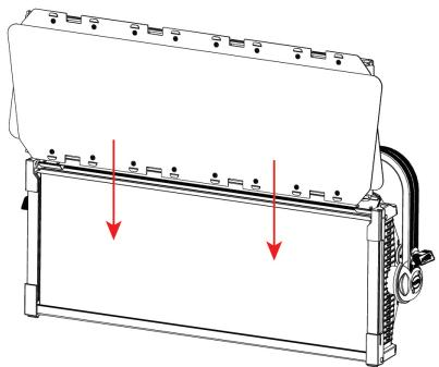
3. With the barndoors locked securely in place, pull on the tabs at the edges of the barndoor flaps to deploy the barndoors. Installation is now complete. Please note that the barndoor accessory must be installed with its own safety cable! Refer to the diagram in the Fixture Installation section of this manual.
