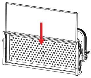
3. Flip the top edge of the fixture frame back down into place, and lock the frame tabs back into place. The installation is now complete.
