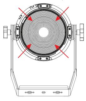
2. Slide the barndoor into the slot in front of the gel frame, then close the gel frame latch to secure in place.
