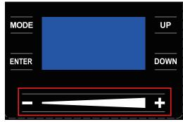
To enter Touch Bar mode, select the TOUCH BAR MODE option from the main system menu, as described in the System Menu section of this manual. Then use the UP and DOWN buttons to scroll through the different modes. Each mode is represented by one of the tables below. Press ENTER to select the mode that is currently dispalyed.
