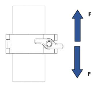
A Do not use fixings that, when tightened, will contact the tube or barrel on which the clamp is fixed as highlighted above.
