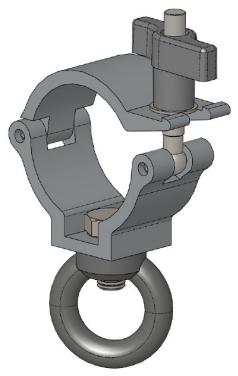
Hanging clamps are commonly used to secure rope directly or via shackles, karabiners, hooks etc.
