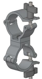
These couplers are used for rigging two sections of truss or barrel together. The couplers consist of two Super Lightweight clamps bolted together and are free to rotate relative to each other. To install, attach each of the clamps that comprise the coupler to their respective barrel or truss following the instructions set out in Sections 10d to 10h.
