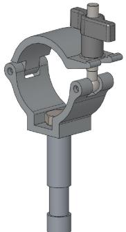
Super Lightweight Beamer Clamps consist of a 16mm beamer spigot fixed to a Super Lightweight clamp. Beamer clamps are commonly fitted into a receiver mounted on a stand. Once the clamp has been inserted into the receiver and locked in to place the barrel or truss can fitted into the clamp following the instructions set out in Sections 10d to 10h.
