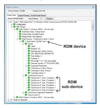
If the user wishes all 6 output channels to be consecutively addressed, this is achieved by setting the RDM device start address (right-click on the RDM device entry). Alternatively, if the user wishes to individually set the address of each channel, this is achieved by setting the start address of each sub-device (right-click on the desired RDM sub-device).
