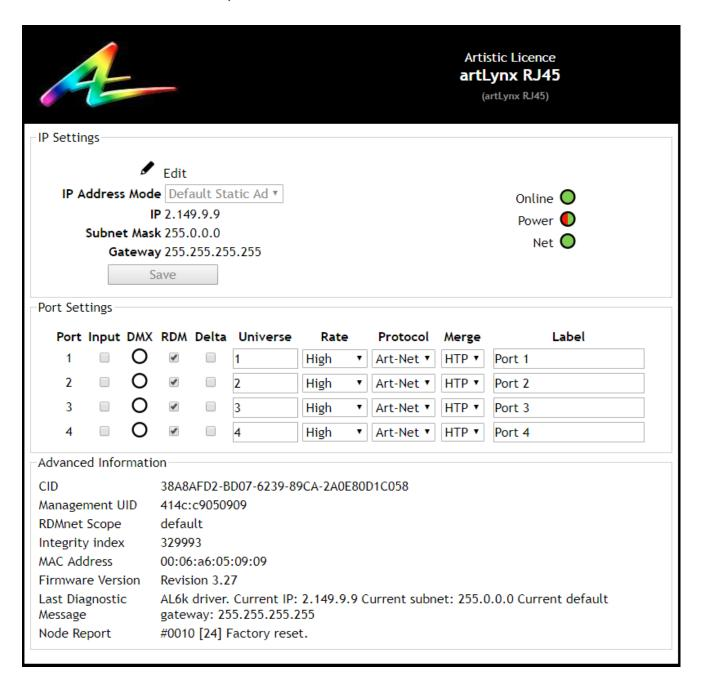
Figure: artLynx RJ45 internal web server
