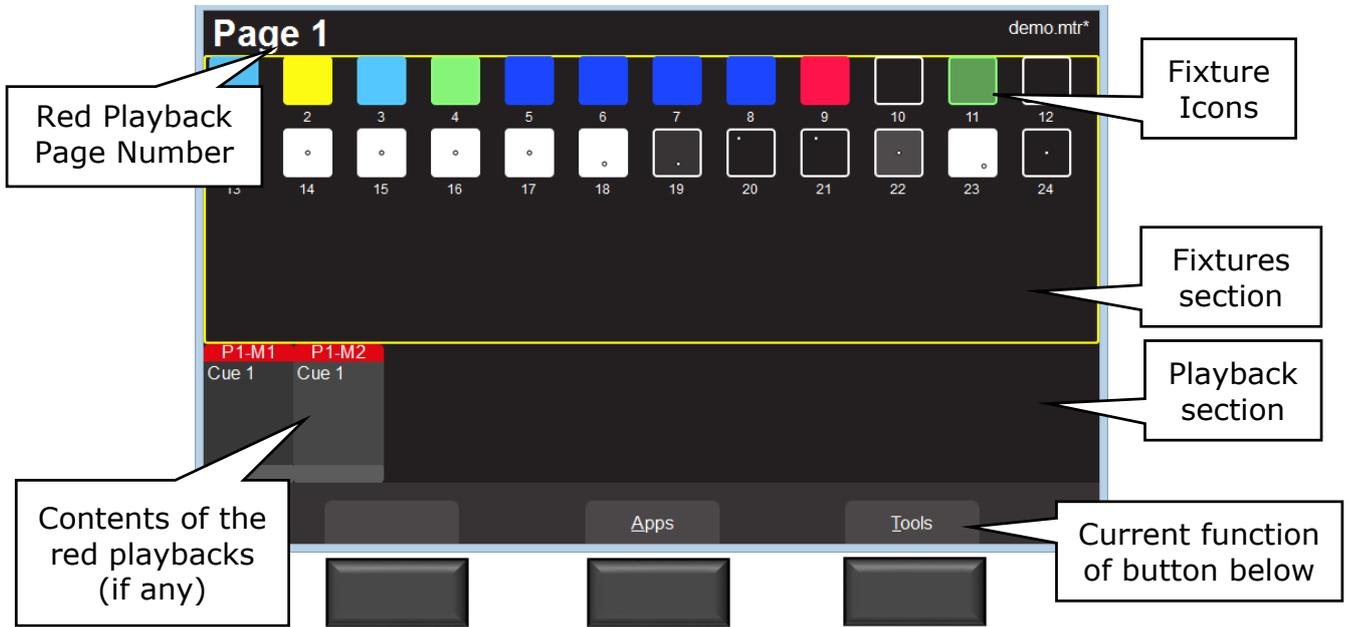
The 3 buttons below the touch screen have different functions for different screens. Their current function (if any) is shown on the screen above each button. You can either tap the button or touch the screen to operate them.
