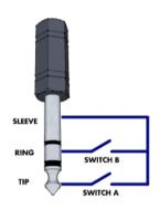
Only use passive pedals that simply short-out the tip & sleeve (Switch A) or ring & sleeve (Switch B) of the  $\frac{1}{4}$ " jack. Do NOT use any proprietary type pedals which do not a standard mono/stereo  $\frac{1}{4}$ " jack connections, or which transmit any additional power or control signals along the cable.
