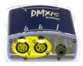
For your convenience the interface has two DMX output sockets, a 3-pin XLR and a 5-pin XLR. This allows you to connect your lighting rig using either 5-pin or 3-pin XLR cables. (Although the official DMX standard specifies 5-pin connections, many lighting manufacturers routinely use 3-pin connections on their most popular lighting fixtures).
