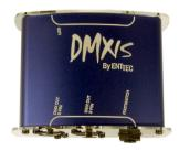
The DMXIS hardware interface is a professional standard USB-DMX converter, capable of transmitting a full universe (512 channels) of DMX-512 data at full 40 Hz frame rate.
