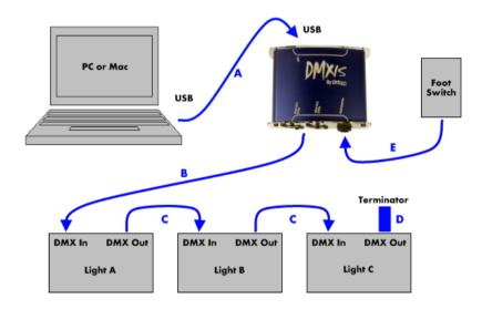
: Connect the DMXIS hardware interface box to your computer with a USB cable.
