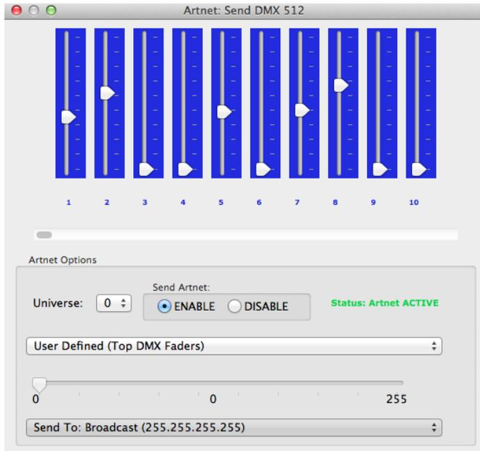
When first opened, the Art-Net is set to Disabled, please set it to Enabled, and then you can use either the DMX faders to test one or more DMX channels, or use the test-patterns from the options available.
