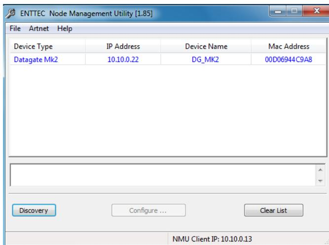
NMU (Node Management Utility) is a free Windows and OSX application that is used to manage compatible ENTTEC DMX over Ethernet nodes. NMU will not directly allow you to configure the Datagate Mk2 itself, but it can help you find your unit's IP address and then open a browser window to make the required changes. To employ the NMU, follow this set of instructions:
