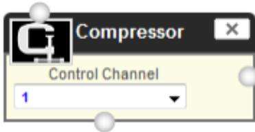
Compressor proportionally reduces all channels of the input according to the value on the control channel. For example: if control value input is 127 all the values on the input will be reduced to 50% at output.
