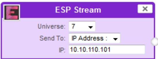
ESP Stream: ENTTEC Show protocol DMX over Ethernet stream (ESP). IP address is the destination address used when the stream is sending data only.
