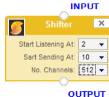
Shifter: can be used to shift a number of channels to another spot in the INPUT DMX frame Channels not defined will be left at 0 value Example: To Shift 100 channels from 10 to 210: Setup as "start listening at": 10 and, "start sending at": 210, "number of channels": 100
