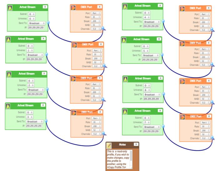
Create a new profile or edit an existing one using the profile-editor. Opens up in a new page in your web browser. Select a module on the left and the right panel will provide help about that panel. Connect a module to another using wires from one point to another. The direction of the wire (arrow) is important, the arrow signifies output, and reflects the flow of data.
