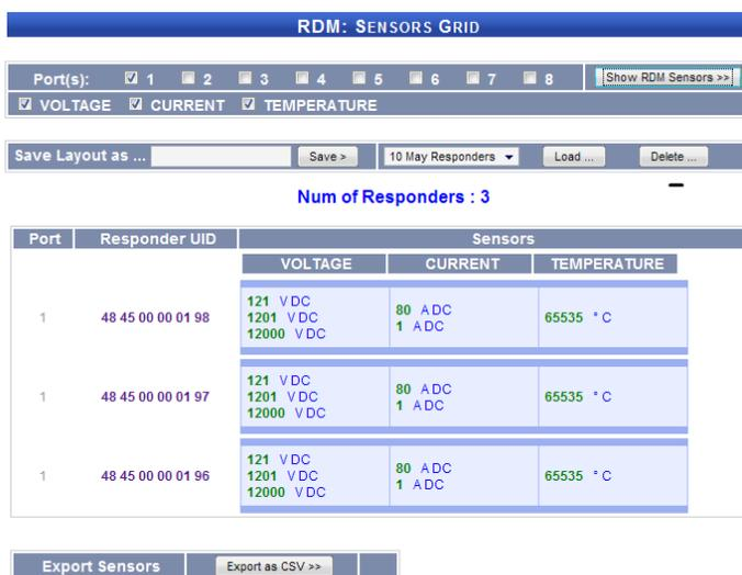
RDM Sensors page, allows discovering all RDM devices and monitoring all sensors supported by the RDM devices found. Examples include: Temperature, Current and, Voltage sensors. The displayed sensors values are refreshed, automatically every few seconds.
