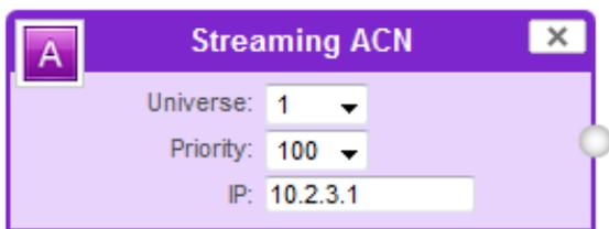
Streaming ACN: "IP address" is the destination address used when the stream is sending data only (default is disabled = 0.0.0.0)
